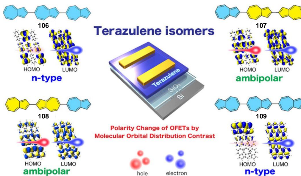
Figure 1.39. Four terazulene isomers and their polarity of OFETs with HOMO and LUMO density distributions [104]
